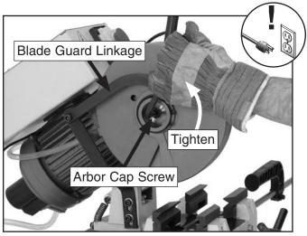
Figure 26. Tightening blade.
